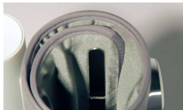
Cuff fabric with embedded metal electrodes that balance between aesthetics and signal accuracy
